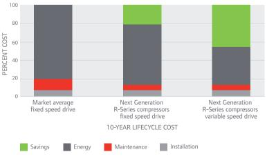
Rotary comparison at 79% average volume capacity; 4000 hours per year; 0.1€/kWh
