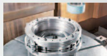
煞車環端面+內外徑研磨
